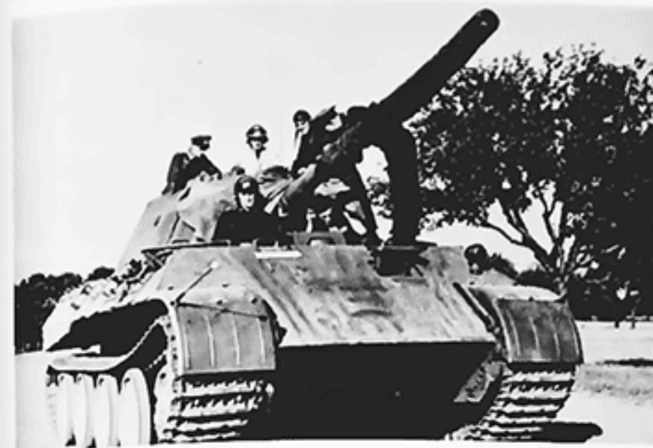
Above: This Panther Ausf D (License Nr. 1A-0805) shown during testing at a proving ground was produced after July 1943. The right Tarnlampe (headlight) and the Verständigungsoeffnung (communications port) in the left turret side had been dropped. A mounting ring for the anti-aircraft machinegun mount was welded onto the commander's cupola. (TTM)
