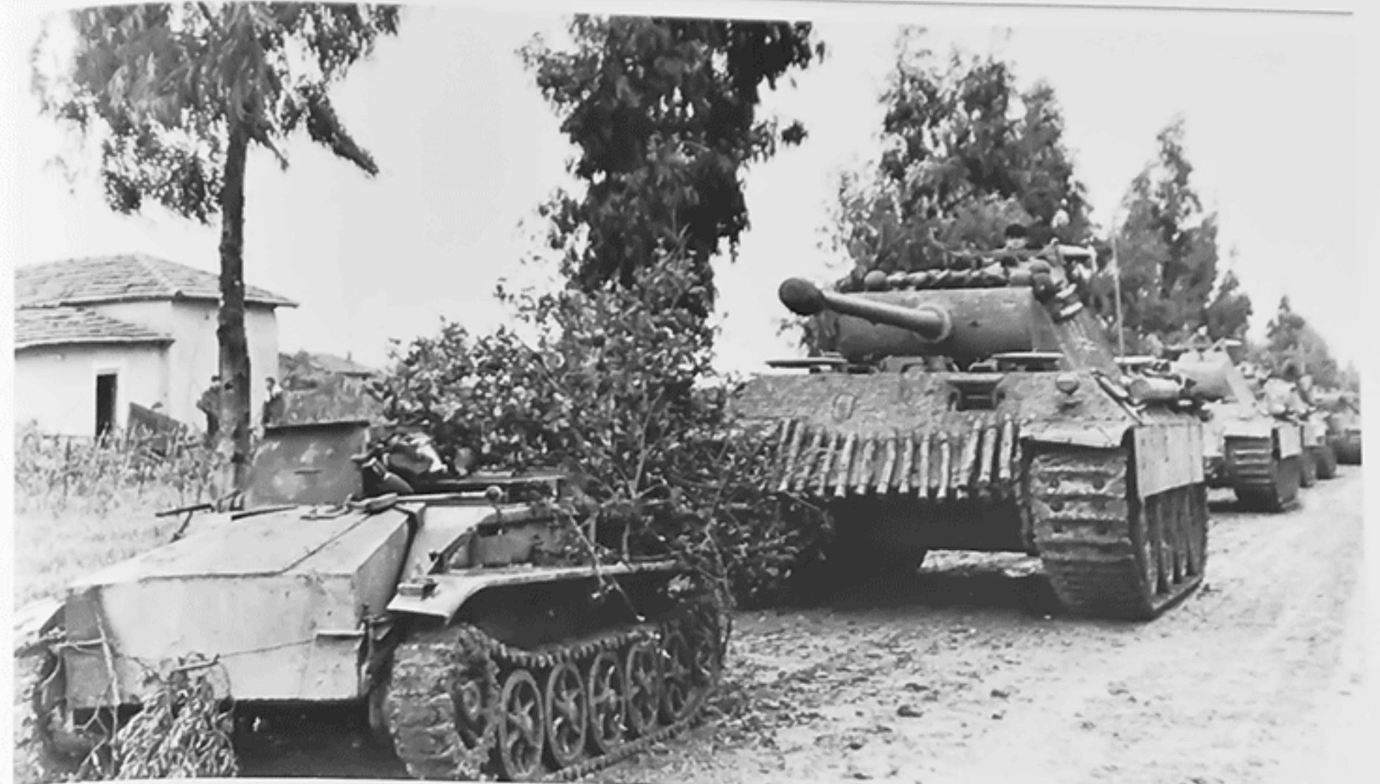
A column of Panthers with the I.Abteilung/Panzer-Regiment 4 waiting to attack at Anzio. Most of the Panthers were Ausf. A with a few Ausf. D. The lead Panther Ausf. A has a monocular T.Z.F.12a gun sight but still has the "Letterbox" machinegun port in the glacis plate. (BA)
