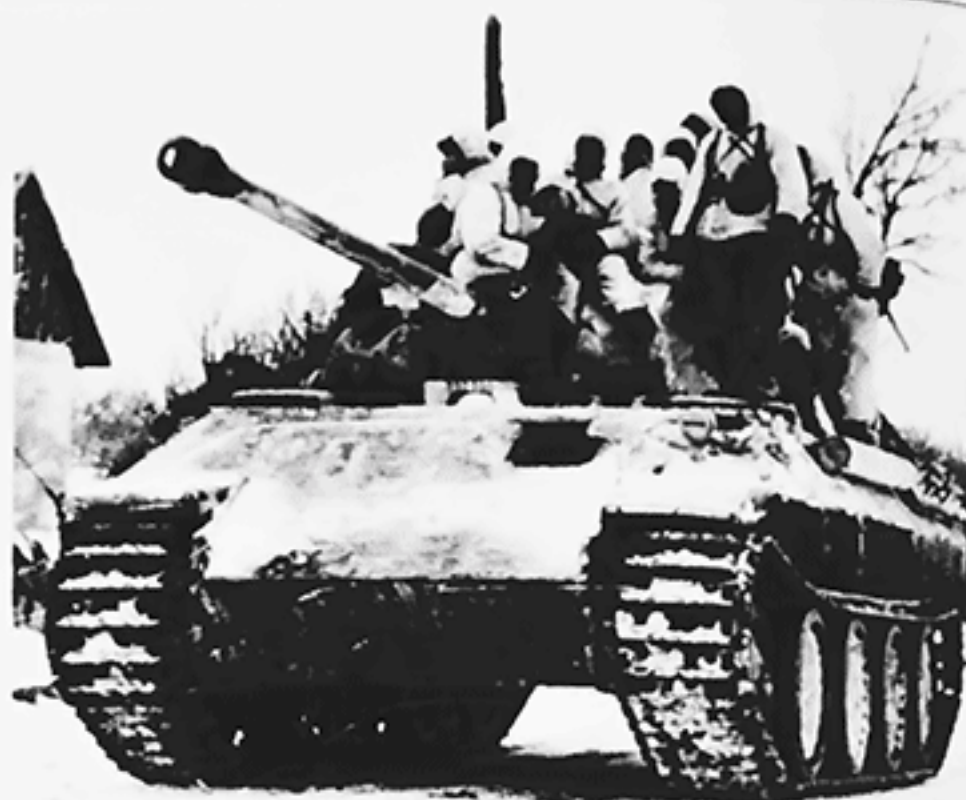
Panther Ausf A (Fgst Nr. 152151 produced by Daimler-Benz on or about 16 December 1943) still has a "Letterbox" machinegun port on the glacis plate. It has a T.Z.F.12a monocular gun sight with a single sight aperture under a wide rain guard. (BA)
