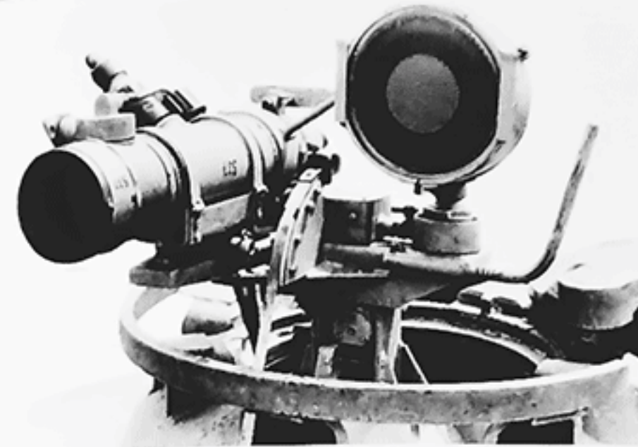
Above and right: The F.G. 1250 infrared searchlight and scope mounted on the commander's cupola of an Panther Ausf. G. The steel band was fed through a hole in the turret roof at the base of the cupola. This steel band, connected internally to an indicator, allowed the gunner to recognize when the elevation of the gun was on target (WJS)
