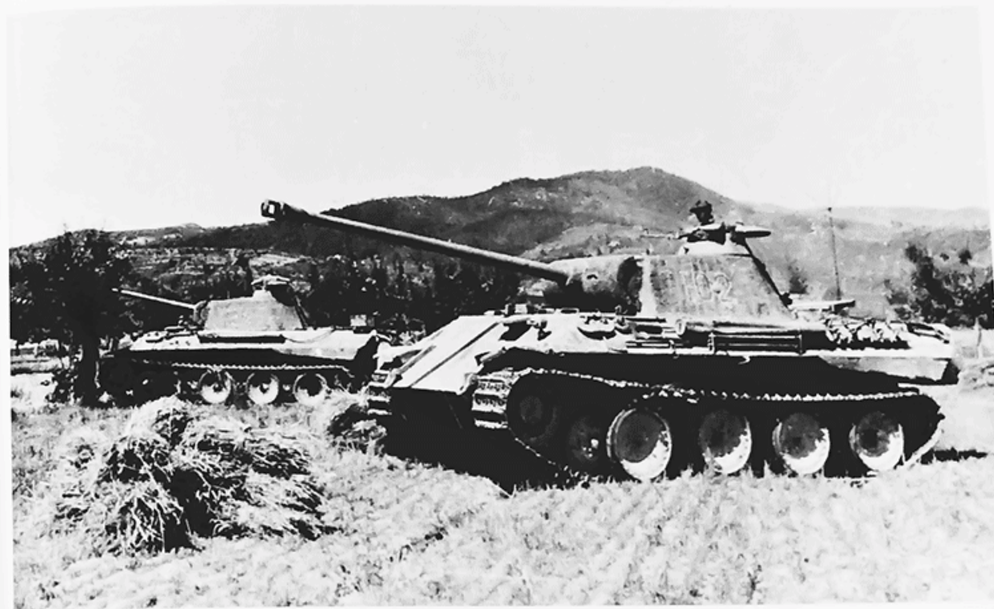
A Befehls-Panther Ausf A, Tactical No. 102, in Italy with the I. Abteilung/Panzer-Regiment 4, still has the T.Z.F.12 binocular gun sight, "Letter Box" machinegun port on the glacis, and pistol ports on the turret sides. As in all Befehls-Panthers, the aperture for the coaxial machinegun was sealed with an armor plug and the spare antenna rods were stored in tubes mounted on the left side. (BA)
