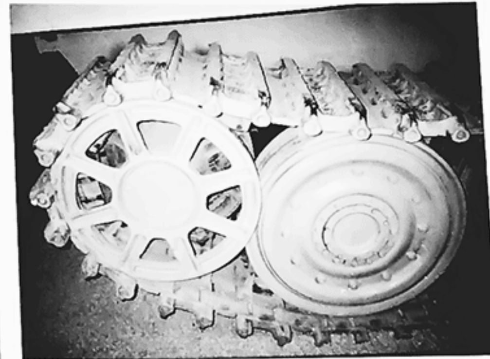
The 660 mm wide combat tracks for the Panther II were to be utilized as transport tracks for the Tiger II. The Gummisparende Laufrollen (Drawing No. 021 D 50204) steel tired, rubber-cushioned roadwheels were specifically designed for the Panther II as was the idler wheel with eight spokes. The drive sprocket was similar (but not identical) to the design used on the Tiger II Versuchs-Serie. (Patton Museum)
