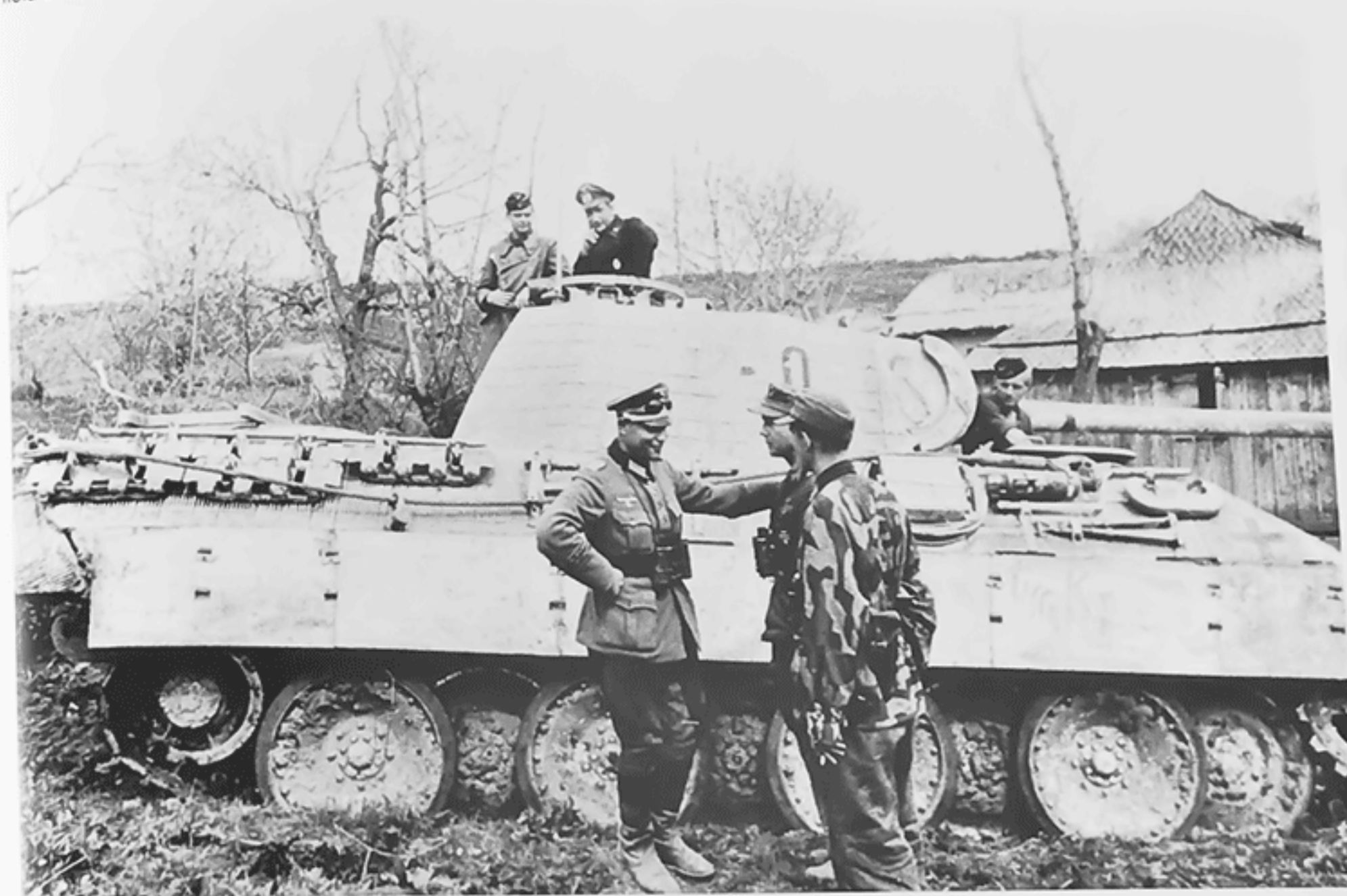
Panther Ausf. A (Tactical No. 231) with the twin pipes parallel to the left exhaust pipe and the jack still mounted horizontally across the engine access hatch. The cylindrical container for the gun cleaning rods has been relocated to a position across the hull rear by the field unit. (BA)
