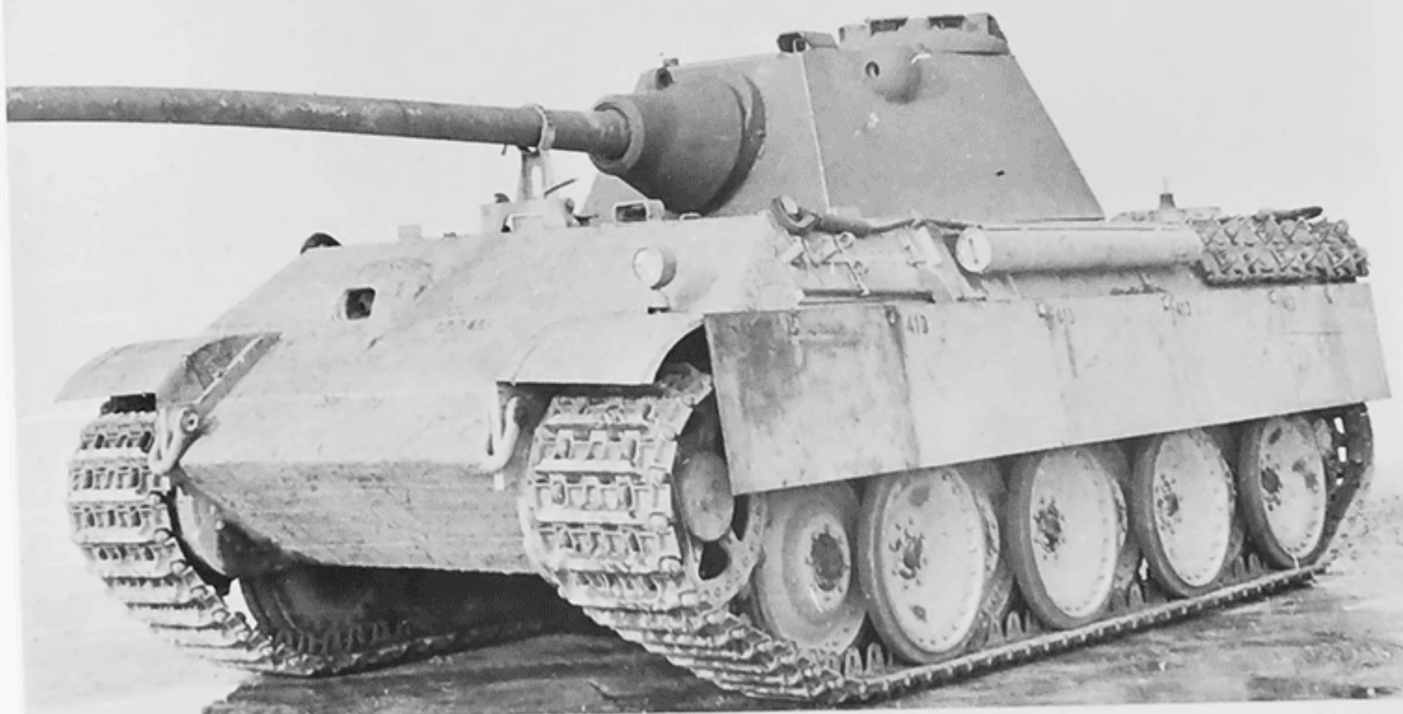
A second Versuchs-Schmalturm mounted on a Panther Ausf.G chassis. The chassis (Fgst.Nr.120413) was completed by M.A.N. for issue to the troops in early May 1944. No hole is evident for a telescopic gun sight in the turret front, only a periscope projecting through the turret roof. The sheet metal debris guard covering the gap between the gun mantlet and the turret front had not been welded on. (WJS)
