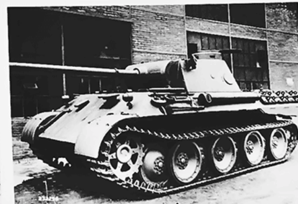
One of the first five Ausf.D Panthers that was assembled by M.A.N. in Nuernberg in January/February 1943. It has the original stowage arrangement for the tools, no rain guards, and no brackets for mounting Schuerzen. (WJS)
