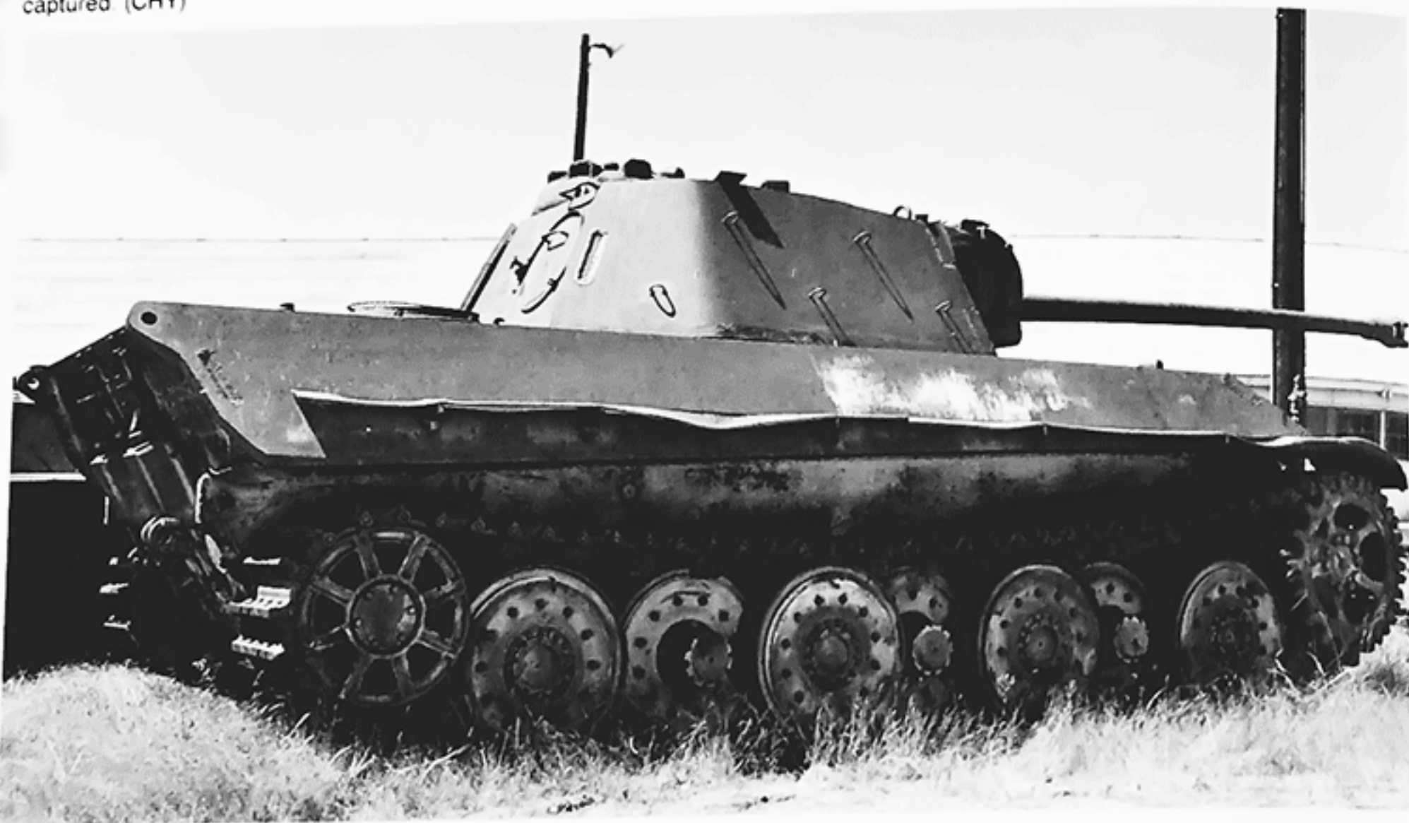
The only chassis completed for the Versuchs-Panther II was captured by the Americans and shipped to Aberdeen Proving Grounds. A Panther Ausf G turret (completed in April 1945) was mounted on the Panther II chassis. It is not known if the turret was mounted by the Germans in a last ditch effort at the end of the War or if Americans mounted an Ausf G turret on the Panther II chassis after it was captured. (CHY)
