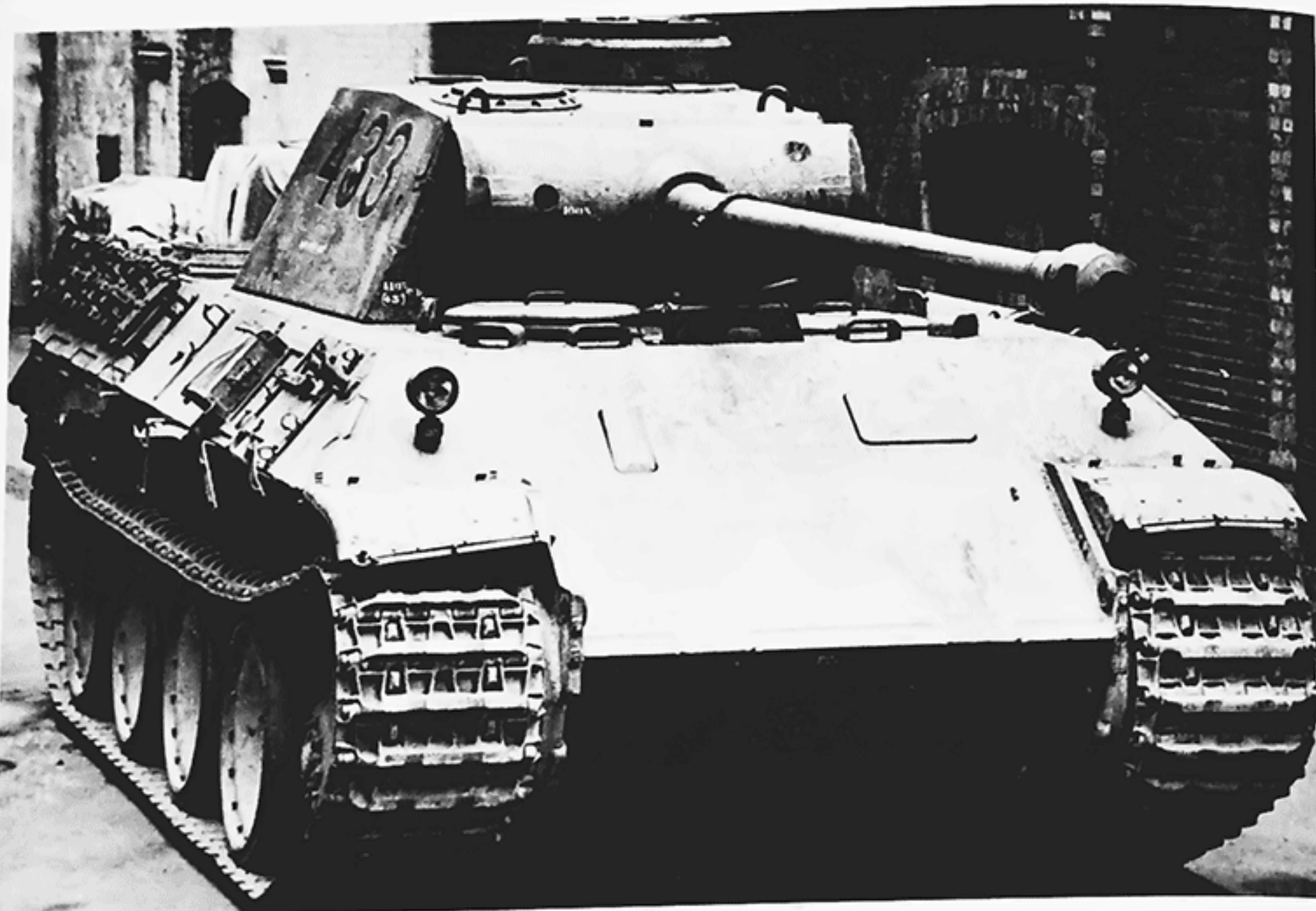
Above and below Panther Ausf D, Tactical Nr. 433 (Fgst.Nr. 213101 completed at M.N.H. in late May/early June 1943) was issued to Panzer-Abteilung 51. It fought at Kursk before being captured by the Russians and shipped to England for detailed examination. Nebelwurfgeraet (smoke candle dischargers) are no longer mounted on the turret sides. Mounting brackets for the track adjusting tool and a sledge hammer have been welded onto the right superstructure side but the jack block is still held by two crossing straps. (NA)
