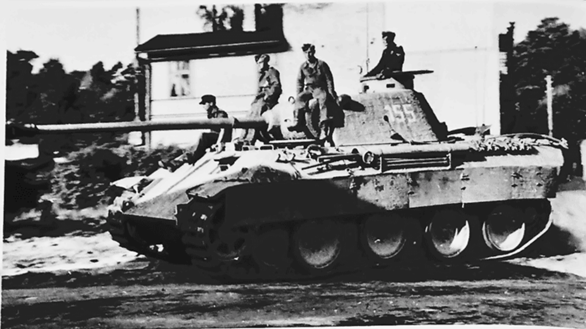
Befehls-Panther Ausf.D, Tactical Nr. 155, possessed the last changes made to Ausf.Ds during production. It had Zimmerit anti-magnetic coating, 24 bolt reinforced roadwheels, and a rain guard over gun sight apertures in the gun mantlet. Replacement antenna rods for the Befehls-Panther were stowed in tubes mounted on the left side below the canister for the gun cleaning rods. (BA)
