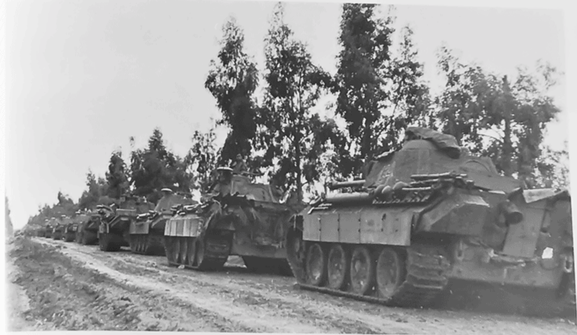
A column of Panthers with the I.Abteilung/Panzer-Regiment 4 waiting to attack at Anzio. Most of the Panthers were Ausf. A with a few Ausf. D. The lead Panther Ausf. A has a monocular T.Z.F.12a gun sight but still has the "Letterbox" machinegun port in the glacis plate. (BA)
