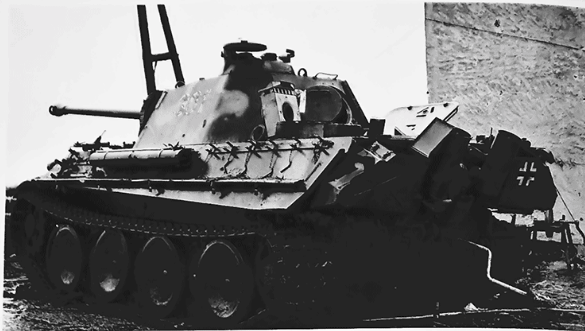
Panther Ausf. G, Tactical No. 301, with a "chin" gun mantlet, without Zimmerit, with Flammvernichter exhaust mufflers, a Kampf-raumheizung crew compartment heater, and larger diameter self-cleaning idler wheels. (NA)
