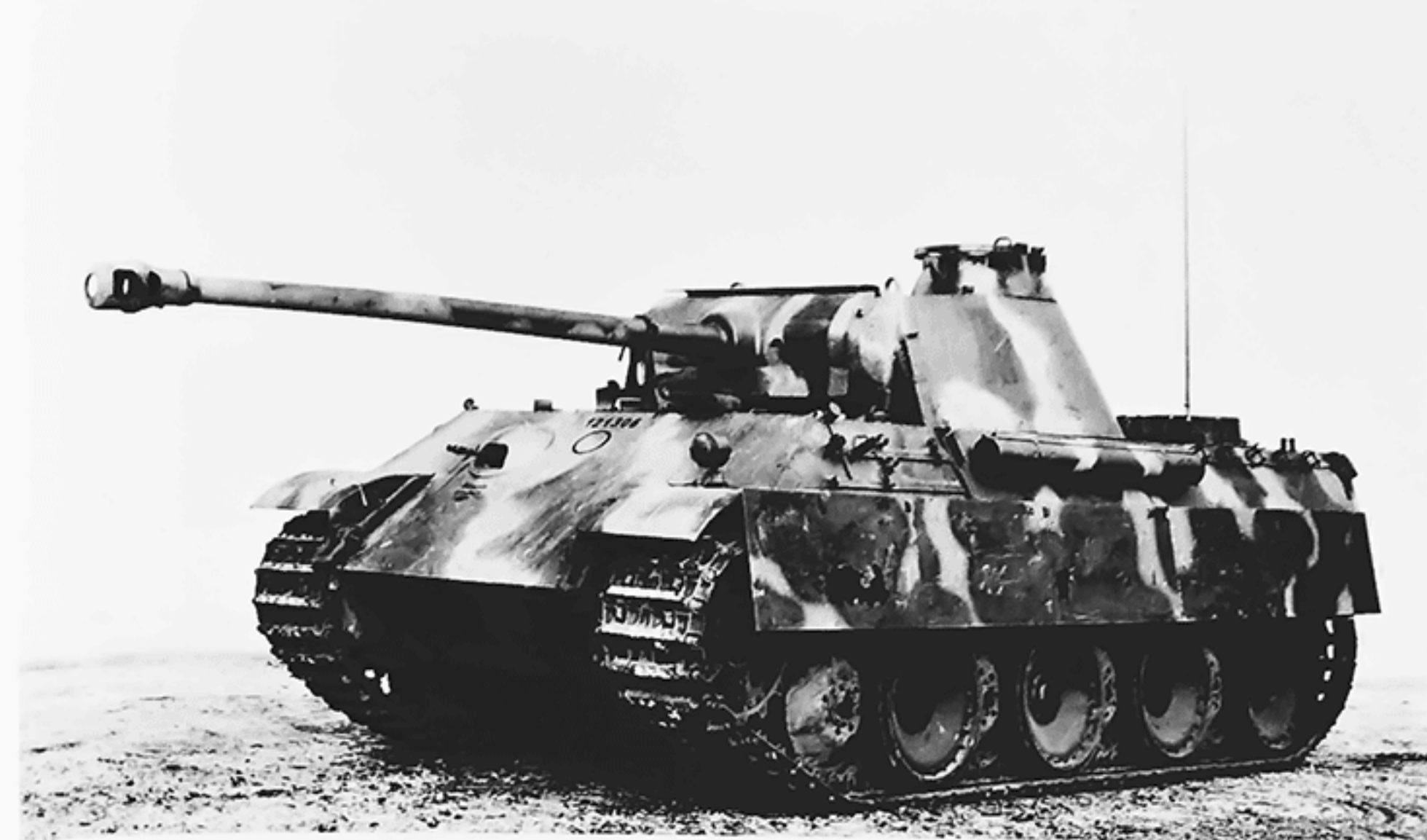
Panther Ausf. G (Fgst.Nr. 121306 completed by M.A.N. on or about 11 December 1944) was tested by Wa Pruef 6. It had a "Chin" gun mantlet and Kampf-raumheizung (crew compartment heater). The cylindrical canister for stowing the gun cleaning rods and spare antenna rods is still on the left superstructure side where it was fastened to all Panthers when they left the assembly plant. (WJS)
