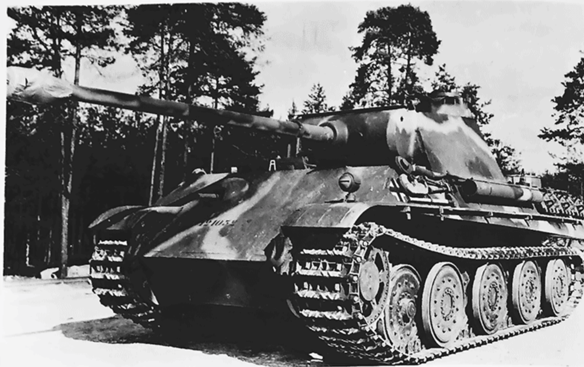
One of the small series of Panther Ausf. Gs (Fgst. Nr. 121052 completed by M.A.N. on or about 22 September 1944) outfitted with steel tyred roadwheels. These roadwheels were the same type used on the Tiger I and Tiger II but were mounted in the normal Panther pattern running on normal Panther tracks. By the time this Panther was completed Zimmerit anti-magnetic coating was no longer being applied. A rain guard has been fitted over the driver's visor. The fan tower on the rear deck was backfitted to this Panther. (NA)
