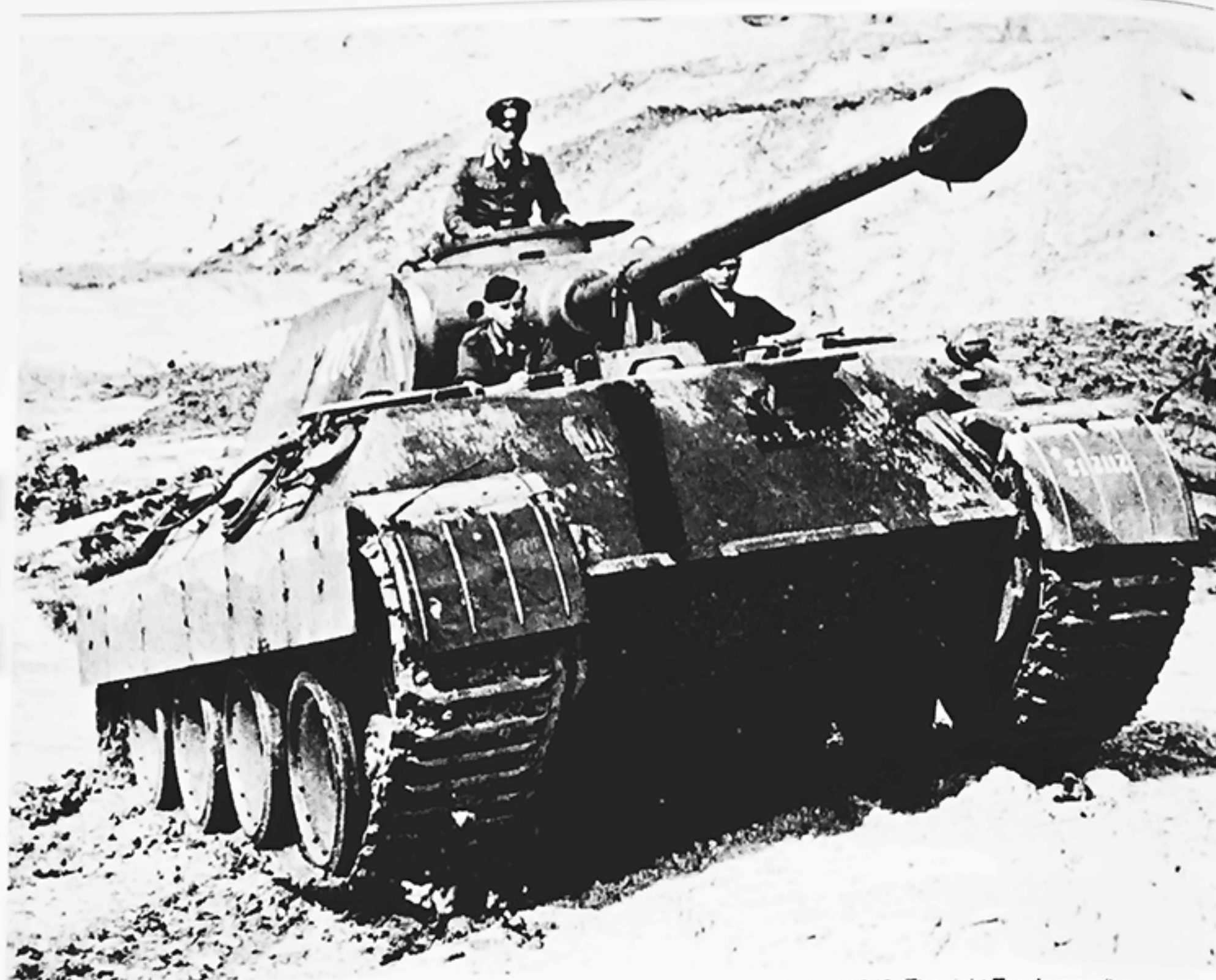
Panther Ausf D, Tactical Nr. 203 (Fgst Nr. 211213) was completed at Daimler-Benz in August 1943. The right Tarnlampe (headlight) has been dropped and a ring for the anti-aircraft M.G. mount was welded onto the commander's cupola. (TTM)
