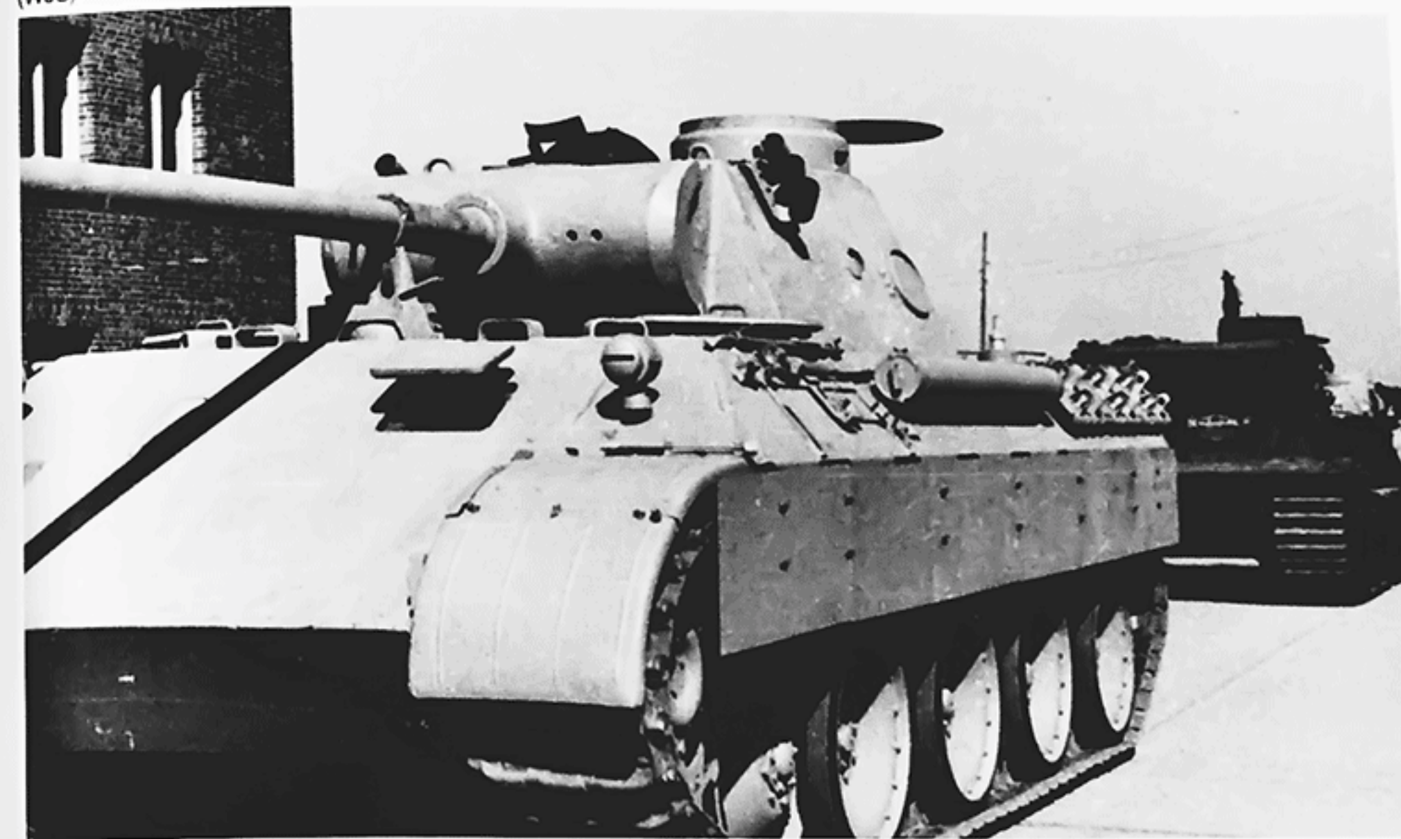
Opposite below and above: These Panther Ausf Ds were completed alongside Tigers at Henschel in early May 1943. They still have Nebelwurfgeraet (smoke candle dischargers) along with the banned rain guards over the pistol port plugs on the turret sides. The opened engine access hatch reveals the pattern used for Maybach HL 210 P30 engines. (HLD)
