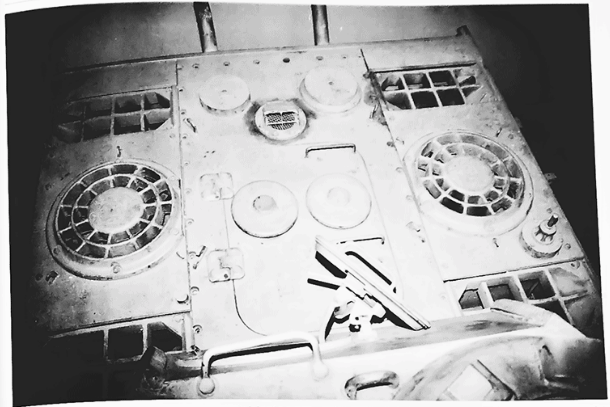
Components on the rear deck (engine compartment air intake scoop, engine combustion air intake covers, and the four rectangular air intake louvers) designed for the Panther II were later adopted into the Panther Ausf G design. The air exhaust louvers covering each fan are the same as those used on the Tiger II. (Patton Museum)
