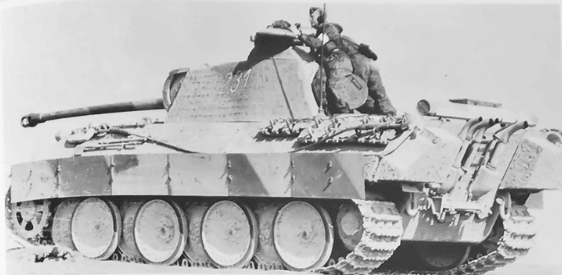
Panther Ausf. A (Tactical No. 231) with the twin pipes parallel to the left exhaust pipe and the jack still mounted horizontally across the engine access hatch. The cylindrical container for the gun cleaning rods has been relocated to a position across the hull rear by the field unit. (BA)
