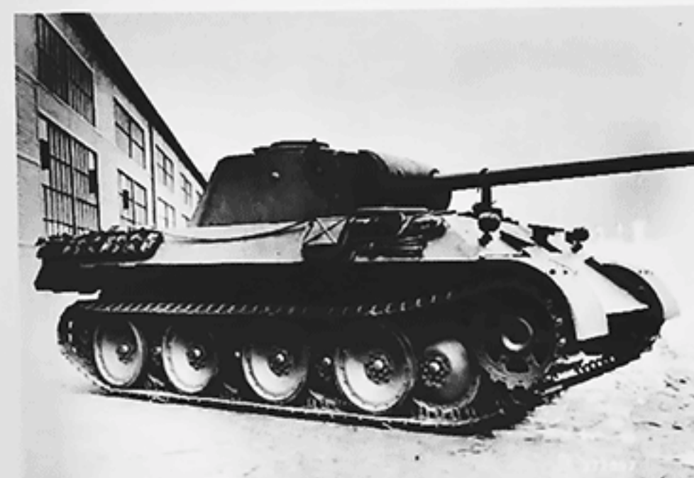
One of the first five Ausf.D Panthers that was assembled by M.A.N. in Nuernberg in January/February 1943. It has the original stowage arrangement for the tools, no rain guards, and no brackets for mounting Schuerzen. (WJS)
