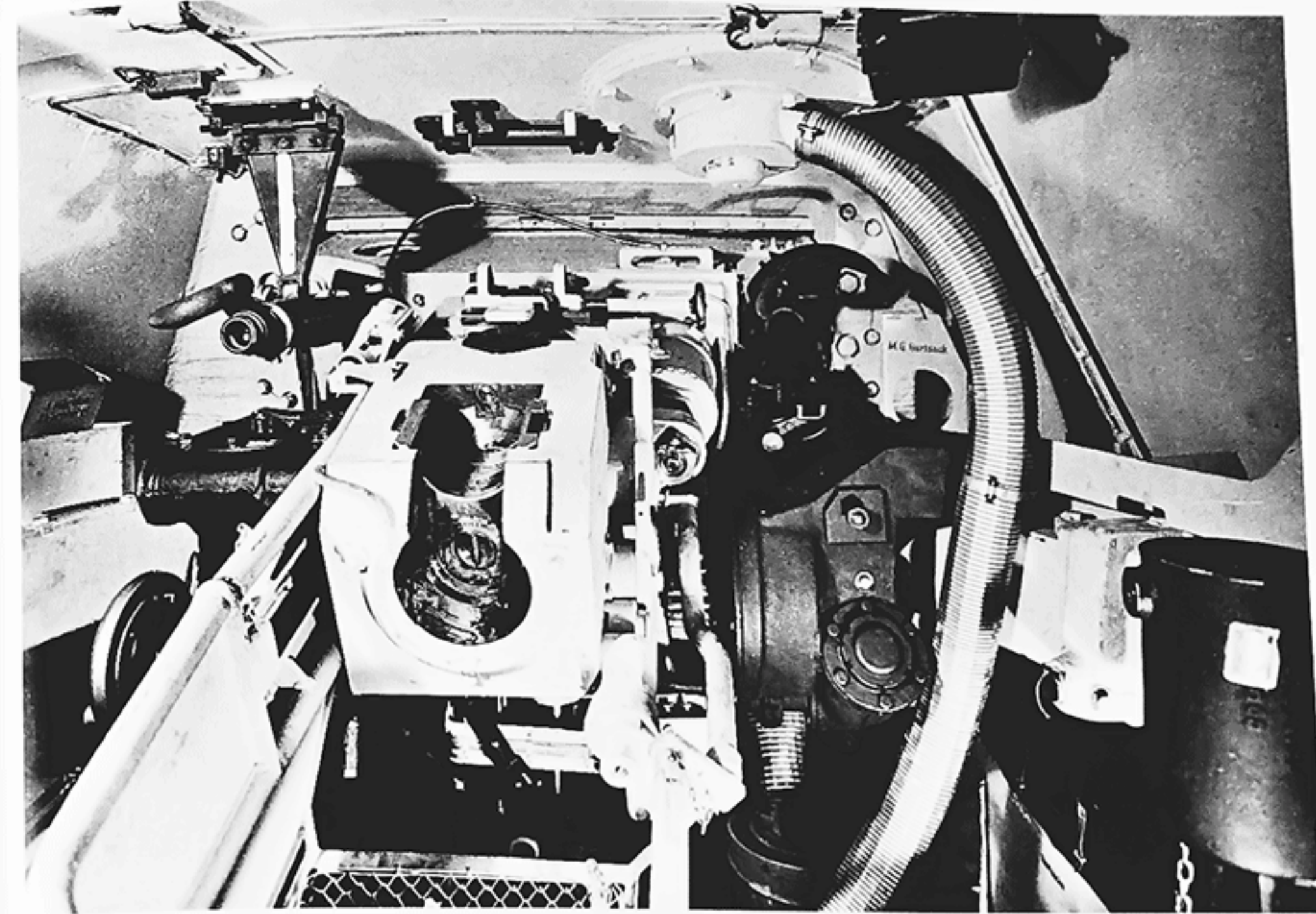
The interior of a Panther Ausf A turret completed in January 1944 with a coaxial machinegun and a T.Z.F.12a monocular gun sight. (WJS)
