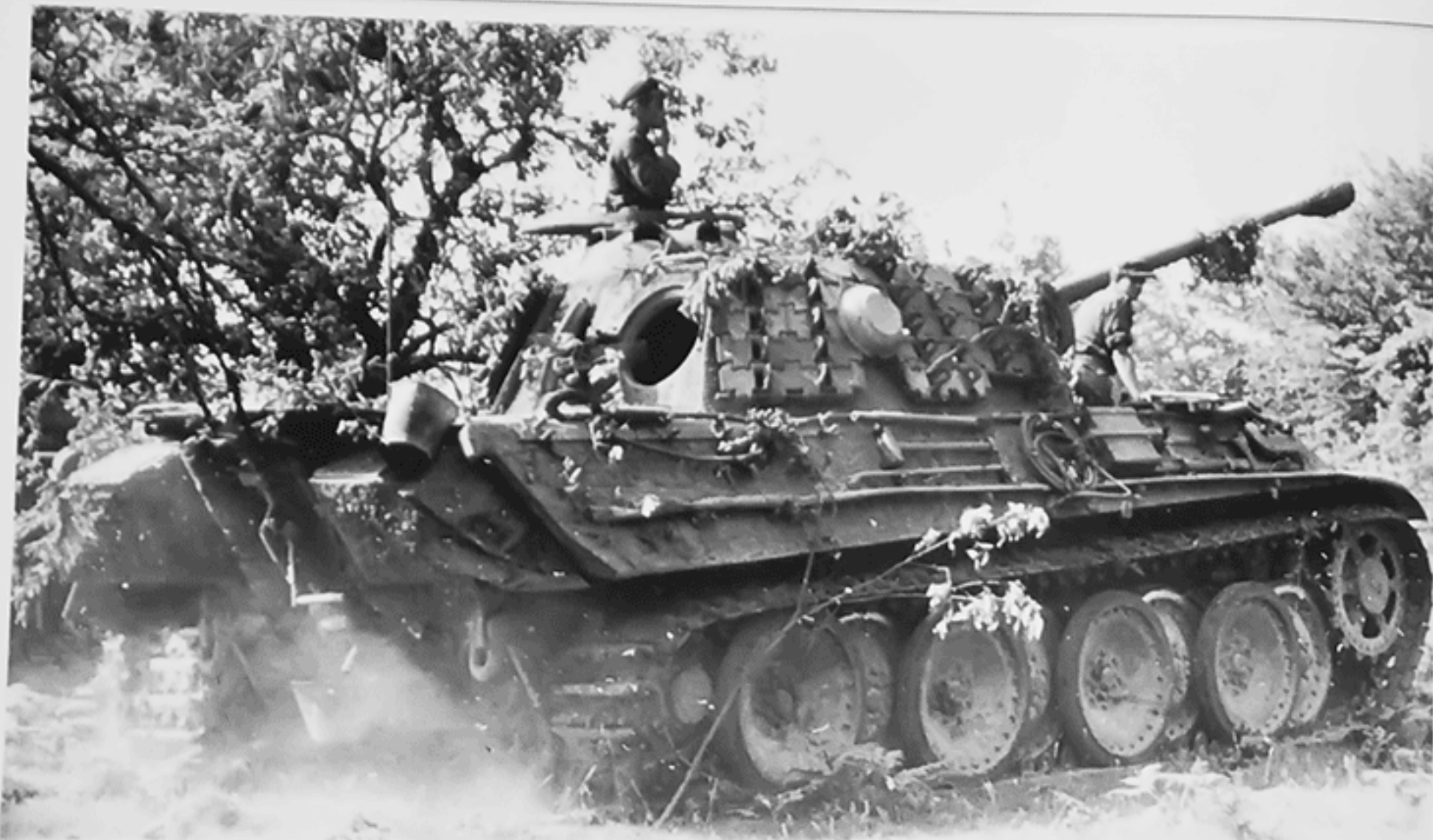
Spare track links have been hung from the turret sides of this Panther Ausf. G in an attempt to increase protection. (BA)
