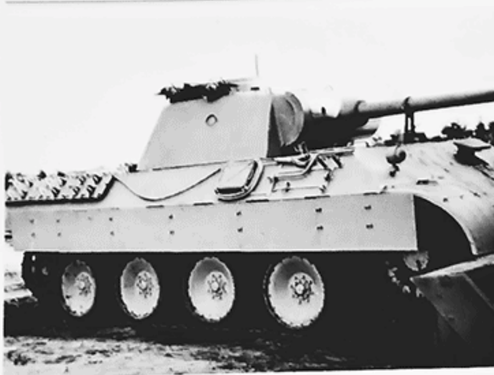
Panther Ausf D (Fgst.Nr. 212061 completed at Henschel in late May/early June 1943) was used in an experiment to test complete submersion. It still has the original stowage layout on the right side and a rain guard welded over the pistol port. (WJS)
