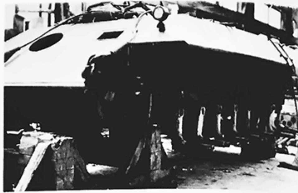
M.A.N. assembled a Panther Ausf A for testing that did not have interlocked armor for the front and side plates. (NA)
