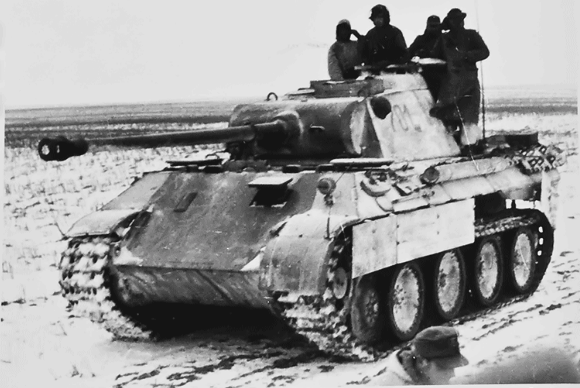
Some of the Ausf.As produced in August and September 1943 did not receive a coating of Zimmerit applied at the factory. Pistol ports are still present on the turret sides and rear along with the binocular T.Z.F.12 . (BA)
