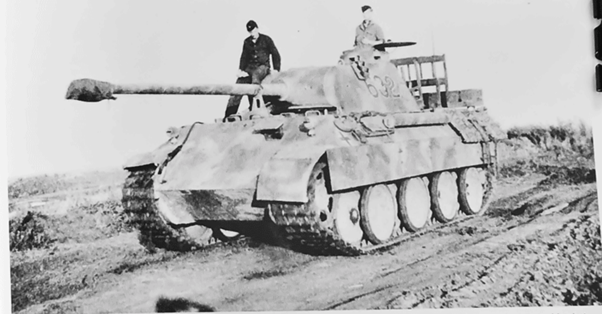
Panther Ausf.D (Tactical No. 632) with Panzer-Abteilung 52. The smoke candle dischargers are still mounted on the turret sides but they are empty. (KHM)
