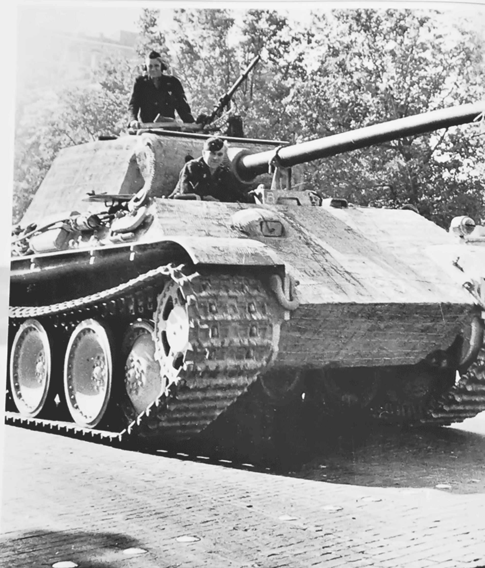
A Panther Ausf. G with the M.G.34 on the cupola prepared for anti-aircraft defense. The hull machinegun wasn't mounted. (BA)
