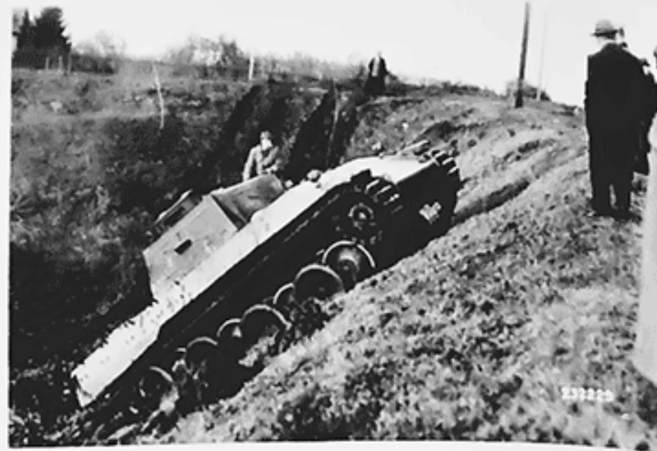
Versuchs-Panther (Fgst.Nr. V1) completed by M.A.N. by September 1942) did not have a turret but was tested with a Belastungsgewicht (test weight). The design of the drive sprocket wheels is unique to the two Versuchs-Panthers. (WJS)
