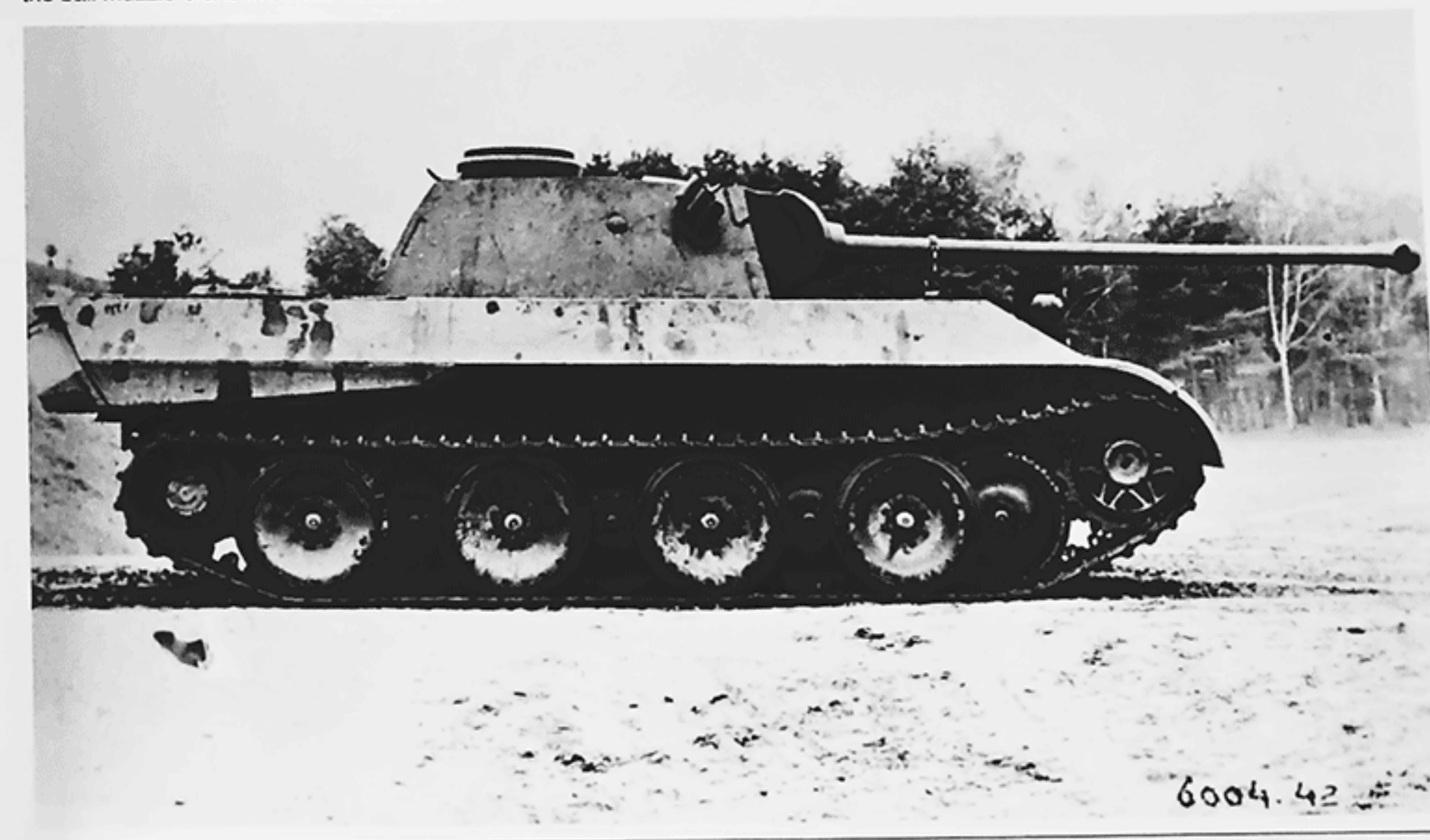
Versuchs-Panther (Fgst.Nr. V2) completed by M.A.N. in the Fall of 1942) was outfitted with a turret. The 7,5 cm Kw.K.42 L/70 still had the ball muzzle brake invented for the 7,5 cm Kw.K.40 L/43 in the Pz.Kpfw.IV Ausf.F2. (WJS)
