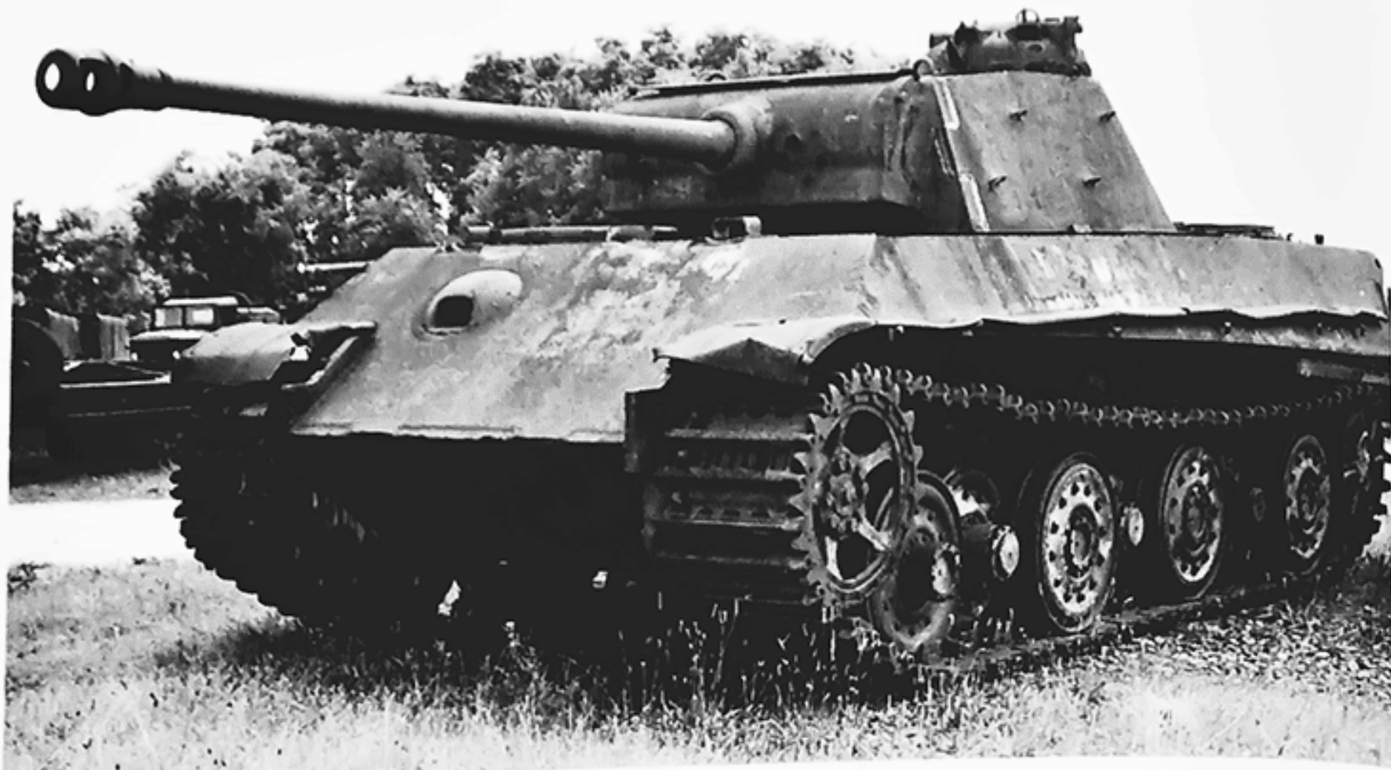
The only chassis completed for the Versuchs-Panther II was captured by the Americans and shipped to Aberdeen Proving Grounds. A Panther Ausf G turret (completed in April 1945) was mounted on the Panther II chassis. It is not known if the turret was mounted by the Germans in a last ditch effort at the end of the War or if Americans mounted an Ausf G turret on the Panther II chassis after it was captured. (CHY)
